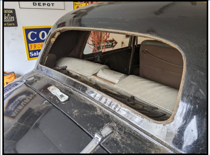
Rear glass and trim removed
