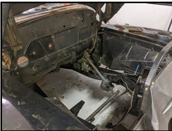
Engine compartment stripped out, too. Only the steering and brakes are left. Front sheet metal loosely reassembled for the body shop.
